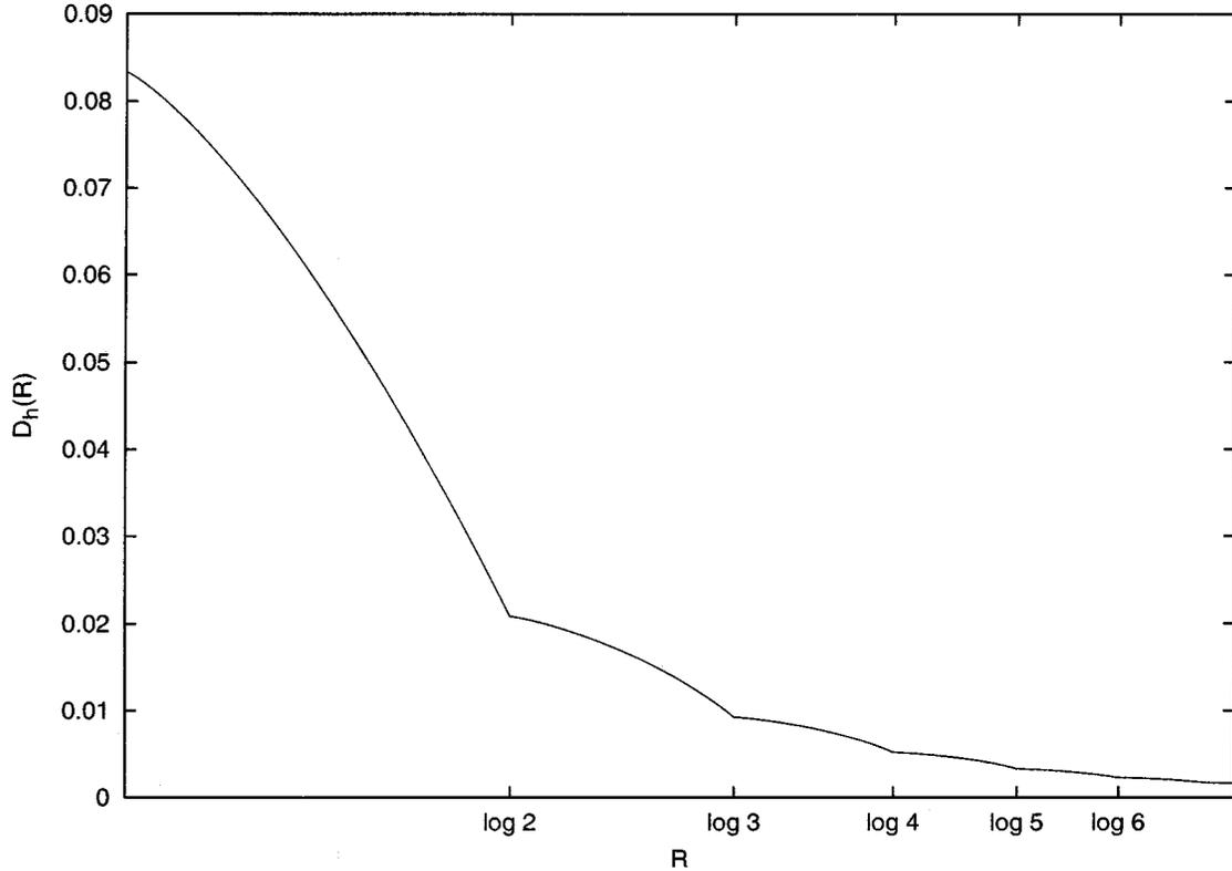
Fig. 1.  $D_h(R)$  for the uniform source and squared error distortion.
